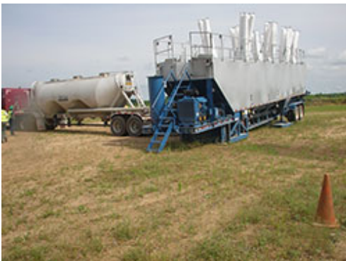
Filter bags of the NIOSH mini-baghouse retrofit assembly (NMBRA) have been installed on the thief hatches on top of this sand mover, used for hydraulic fracturing.
